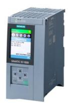
SIMATIC S7-1500F, CPU 1515F-2 PN, central processing unit with work memory 750 KB for program and 3 MB for data, 1st interface: PROFINET IRT with 2-port switch, 2nd interface: PROFINET RT, 30 ns bit performance, SIMATIC Memory Card required
